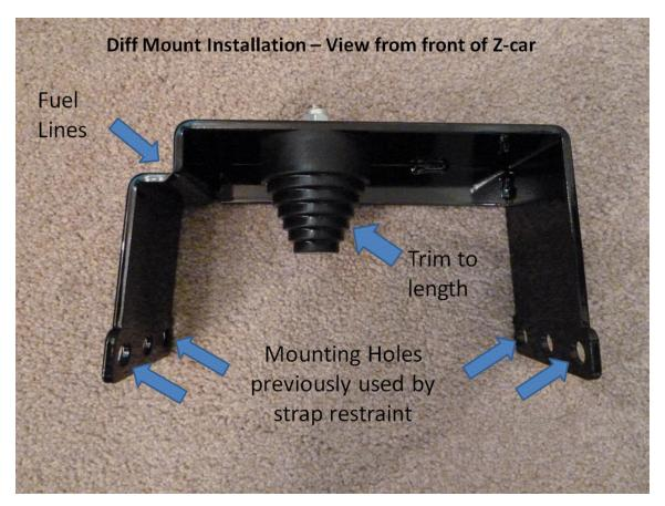
Measure the distance from the bottom of the diff mount to the top of the differential, and trim the snubber to the length you have measured. It can be cut with a hack-saw, or grinder. In
