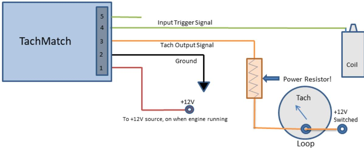
A Vintage Tach is connected this way – remember the need for a ground wire from the negative terminal of the tachometer (**Note:** to prevent damage to your tachometer, don't install the wire to the tach until the jumper, calibration potentiometer and cyl-switches are set as described on the following pages):
