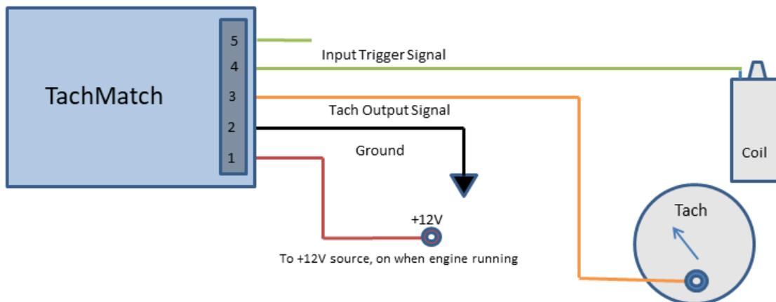
A current-driven tachometer is connected this way:
