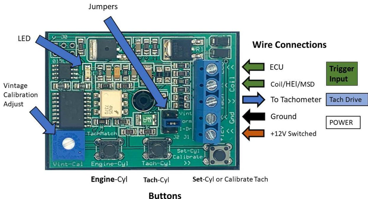
The LED illuminates when power is applied, but goes out when the engine is running, as an indication that triggering is occurring. It is also used for setting the engine and cylinder count.
